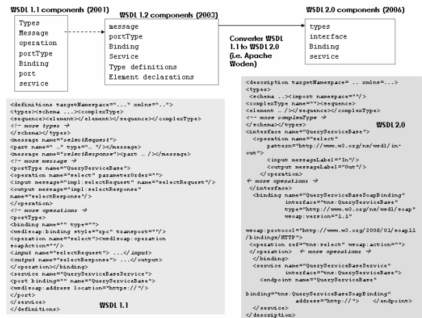
Figure 4. A comparison between the versions 1.x and 2.0 of the WSDL document for the same service (QueryService) making queries to a database that supports the select operation.
